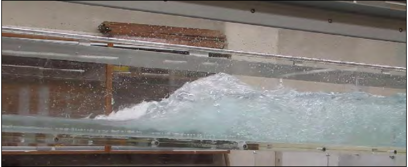
Figure 3 - A hydraulic jump in the lab. Flow moves toward the right.
